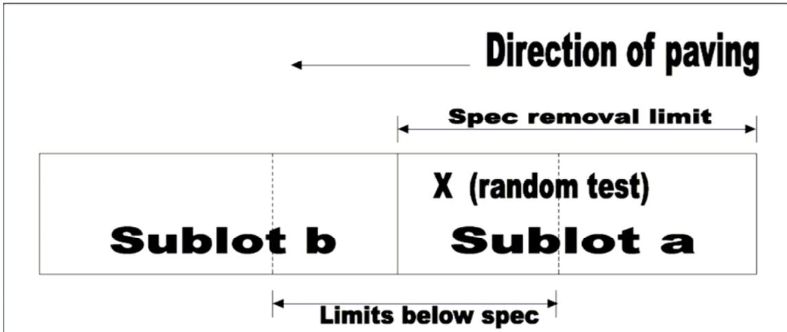
In this example the random QC sample fell late in subplot a and test results indicated that voids were below the limits for removal. By specification subplot a should be removed.
