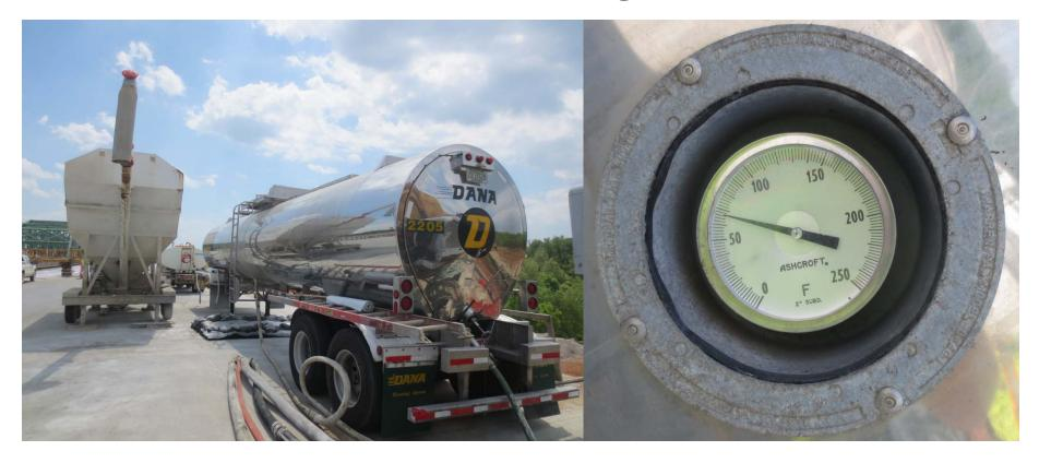
**505.20.2.3** Latex admixture shall be kept in a suitable enclosure that will protect the admixture from freezing and from exposure to temperatures in excess of 85 F. Drums of latex admixture to be stored at the work site in direct sunlight shall be completely covered with a suitable insulating blanket material to maintain an <u>enclosed temperature below 85 F</u>.
