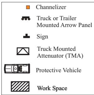
A protective vehicle **shall** be used when work is in progress. The protective vehicle **shall** be equipped with a TMA and flashing arrow panel at least 150 ft. in advance of the work space.
