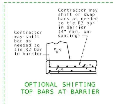
Included on std dwg, but also available as a cell in CADD Std: Optional Shifting Top Bars at Type D or H Barrier (Slab Sheet Details)
