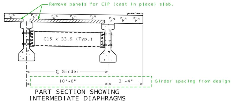
PART SECTION SHOWING INTERMEDIATE DIAPHRAGMS
