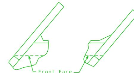
Barrier curb at end bent extends past front face of end bent on skewed structures.
