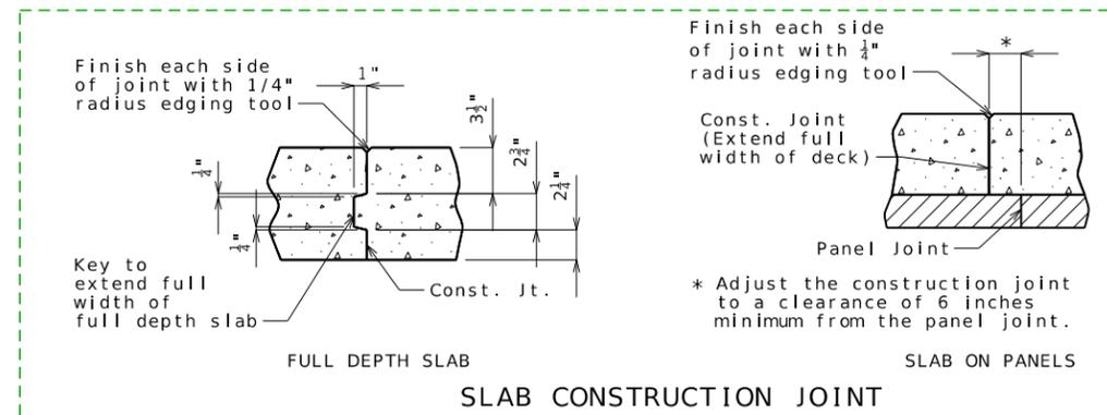
Included on std dwg, but also available as a cell in CADD Std: Const. Joint Detail - P/C P/S Panel Deck (Slab Pouring Sequences)
