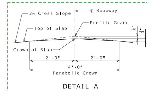
Included on std dwg, but also available as a cell in CADD Std: Parabolic Crown Detail - 2% Slope (Slab Sheet Details or End Bents)
