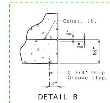
Included on std dwg, but also available as a cell in CADD Std: Drip Groove & Chamfer Detail (Slab Sheet Details)
