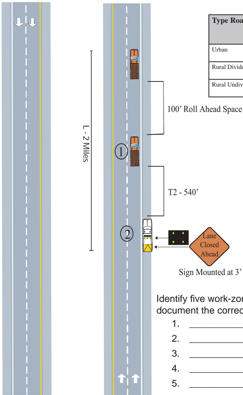
Identify five work-zone errors in the diagram and document the corrections on the lines below.
