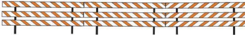
(Typical installation of Type III Barricade with 12' lane no shoulder)
