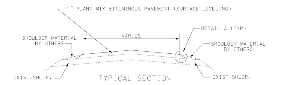
NOTE: SURFACE PLACEMENT SHALL BE ONE PASS PER LANE NO S.E. CORRECTION.
