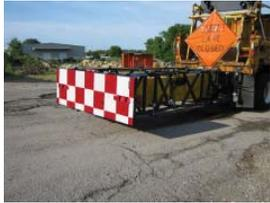
The National Cooperative Highway Research Project tests and sets crash criteria for TMAs and has approved two types of TMA devices: the **230 and 350**. **Only 350-tested units can be used on MoDOT construction projects. MoDOT crews can continue to use both types on the state highway system, but the 230 TMAs can only be used on minor routes. The 230 units are to be marked “for use on minor routes only” and must be relocated to maintenance areas that maintain a large proportion of minor routes.**
