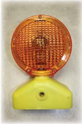
Type A are low-intensity, flashing light units capable of being visible from a distance of 3000 ft. on a clear night. These units may be used during nighttime hours to warn motorists they are approaching or proceeding through a potentially hazardous area. Their use is limited to supplementing other traffic control devices throughout the temporary traffic control zone. They are not be used for delineation.
