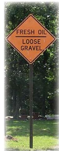
**A minimum lateral clearance of two ft.**, measured horizontally from the edge of the sign to the edge of the roadway, is recommended for installations on roadways with **curbed sections**.
