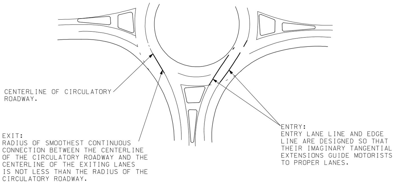
Vehicle Path Overlap at Two-Lane Roundabouts.
