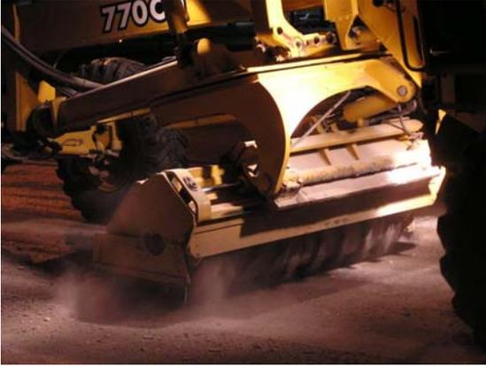
(1) Roto Grader Milling a Pavement Joint
