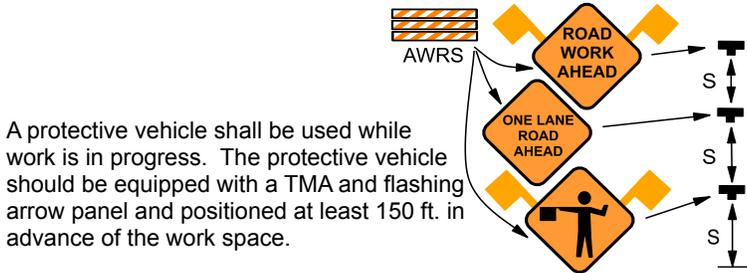
A protective vehicle shall be used while work is in progress. The protective vehicle should be equipped with a TMA and flashing arrow panel and positioned at least 150 ft. in advance of the work space.
