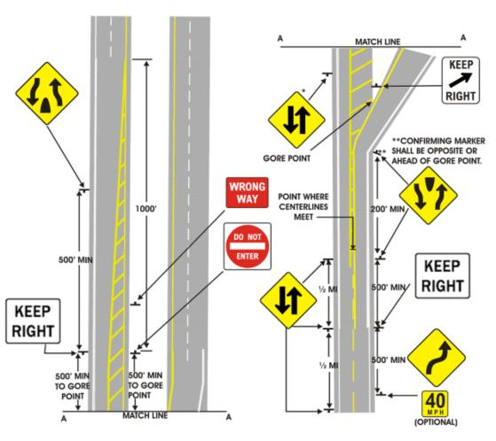
\*TWO ADDITIONAL "TWO WAY TRAFFIC" SIGNS SHALL BE PLACED AT 3 MILES AND 5 MILES FROM THE POINT WHERE THE TWO CENTERLINES MEET (OR END OF DIVIDED HIGHWAY) WHEN THE FOLLOWING CONDITIONS EXIST.
