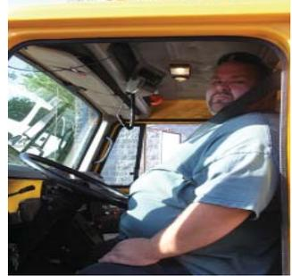
Properly adjusted seat belts may minimize or reduce injuries. A seat belt should be secured in the manufacturer's locking device and should be snug across the chest, not under armpit.
