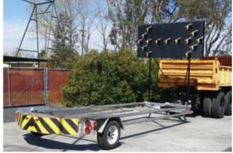
The easy to own and operate Vorteq TL-3 Trailer TMA is lightweight and attaches to most host vehicles with a 20 ton pintle hook and 7 pin electrical connector. Acceptable host vehicle weight is 9960 lbs. to infinite weight. Super fast attachment means you have full TMA protection in less than a minute. The open frame design means inspection and maintenance is quick & easy.
