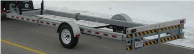
The TTMA-100's rear impact plate is designed to capture the front of a vehicle such that, the trailer becomes locked between the impacting vehicle and the support truck. The pintle hook connection allows the trailer to rotate to remain aligned with the impacting vehicle.
