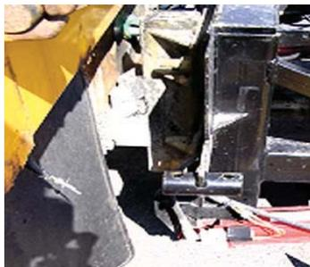
2. Be sure all persons and objects are clear before raising or lowering the TMA. Be sure the system is stopped and in full up position with safety chains securing the unit before allowing anyone to walk behind it.
