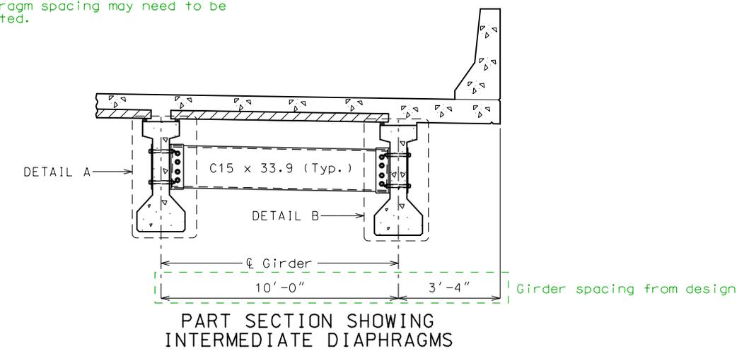
**PART SECTION SHOWING INTERMEDIATE DIAPHRAGMS**
