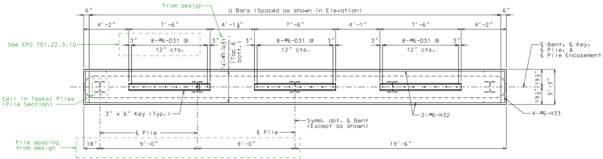
Cell in Tasks: Intermediate Bents (Section thru Key)
