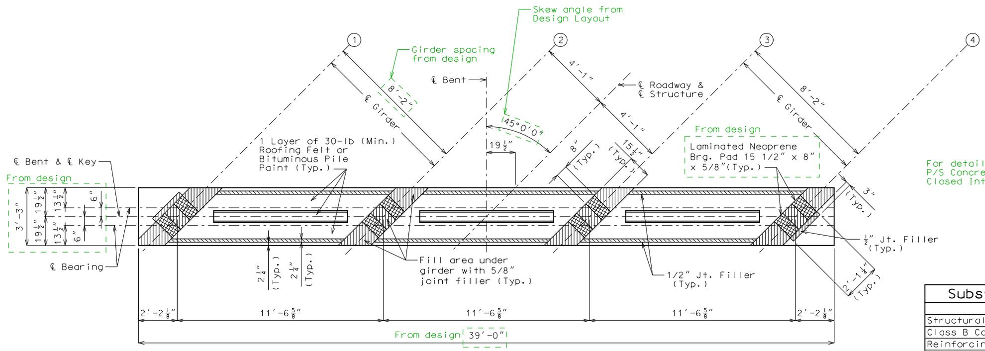
For details of joint filler, see EPG 751.22.3.10, P/S Concrete I Girders, Closed Intermediate Bent Diaphragms
