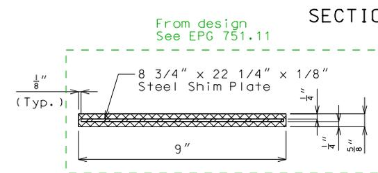
SECTION THRU LAMINATED NEOPRENE BEARING PAD
