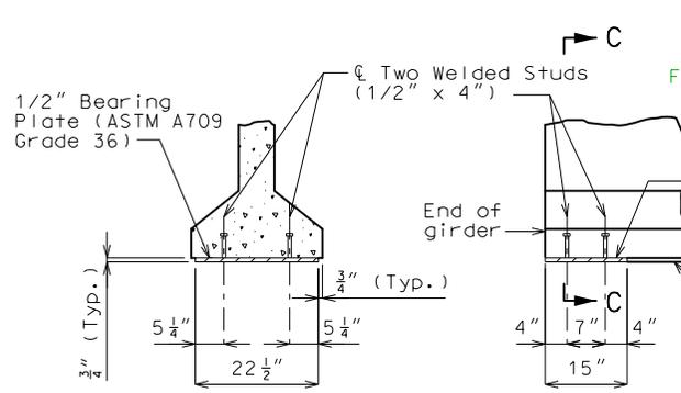
SECTION C-C BEARING PLATE DETAILS and PART ELEVATION AT END OF GIRDER
