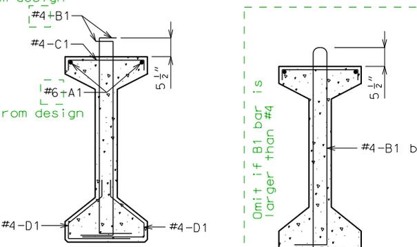
SECTION B-B and B1 BAR PERMISSIBLE ALTERNATE SHAPE
