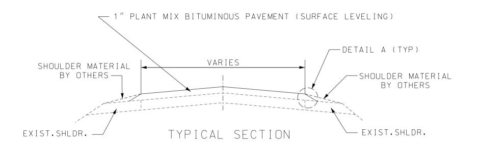
NOTE: SURFACE PLACEMENT SHALL BE ONE PASS PER LANE NO S.E. CORRECTION.
