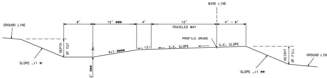
SECTION ON SUPERELEVATED CURVE
