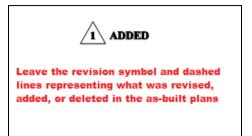
Do not delete, mark through, or alter the revision marks on the plan sheets. Those "marks" are part of the contract plans and need to remain on the plan sheet(s).
