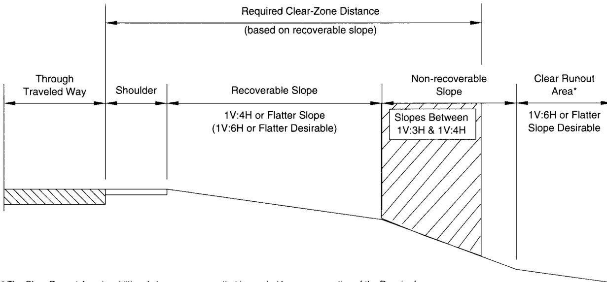
\* The Clear Runout Area is additional clear-zone space that is needed because a portion of the Required Clear Zone (shaded area) falls on a non-recoverable slope. The width of the Clear Runout Area is equal to that portion of the Clear Zone Distance that is located on the non-recoverable slope.
