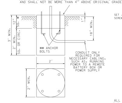
\* SURFACE OF BASE TO BE CONSTRUCTED SQUARE FOR A DEPTH OF 12"
