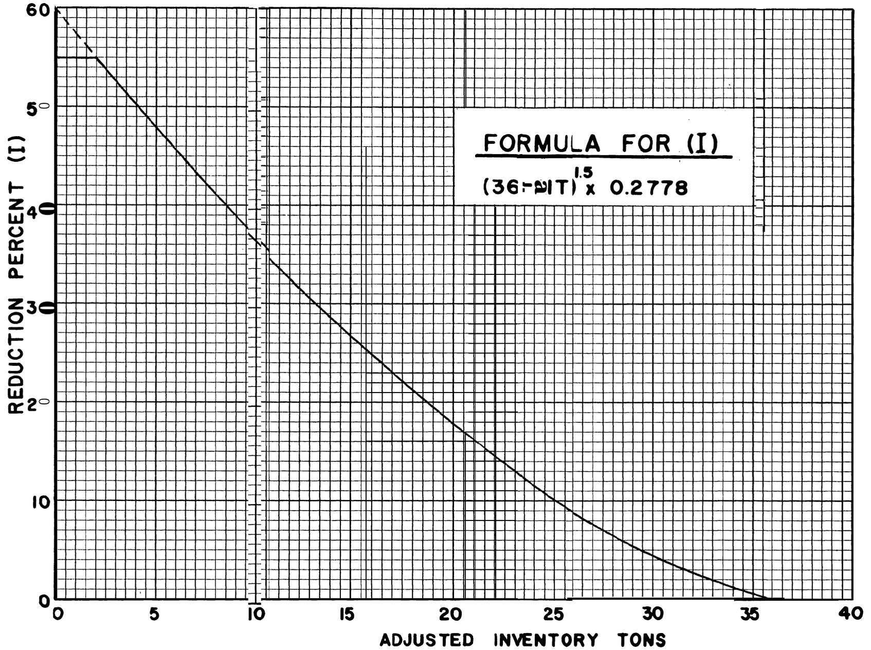
Figure 2. Reduction for adjusted inventory tons
