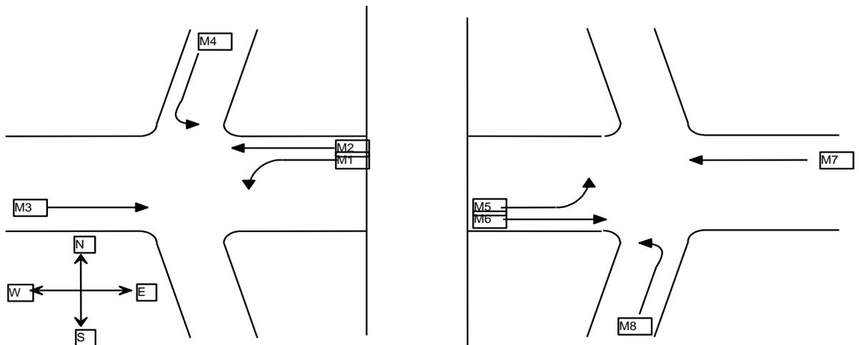
At this interchange, the left turns onto the ramps are protected/permited, with the protected lefts leading along with the first through movement at each end.
