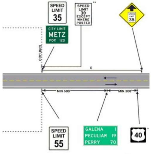
(X)--SPACING INFORMATION CAN BE FOUND IN THE APPROPRIATE EPG ARTICLE. THE SPACING SHOULD BE SUFFICIENT TO ALLOW THE AVERAGE MOTORIST TIME TO DECELERATE TO THE POSTED SPEED.
