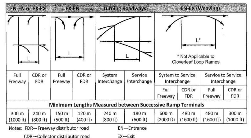
Figure 10-68. Recommended Minimum Ramp Terminal Spacing
