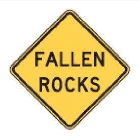
Only used for locations where rock may fall onto the roadway or adjacent shoulder, not for locations where fallen rock is retained in the ditch outside of the shoulder
