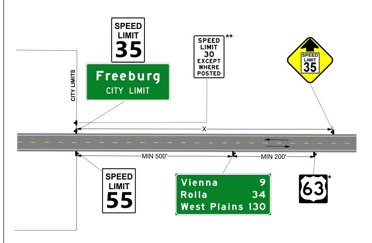
(X)--SPACING INFORMATION CAN BE FOUND IN EPG TABLE 903.6.6 GUIDELINES FOR ADVANCE PLACEMENT OF WARNING SIGN. THE SPACING SHOULD BE SUFFICIENT TO ALLOW THE AVERAGE MOTORIST TIME TO DECELERATE TO THE POSTED SPEED.
